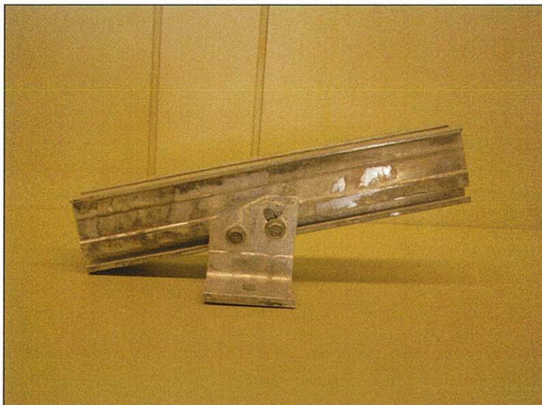
Picture 10: Sample 2 after the treatment with sulfur dioxide and salt mist
