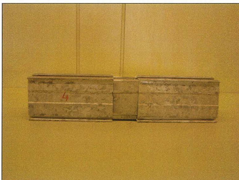
Picture 11: Sample 4 after the treatment with sulfur dioxide and salt mist
